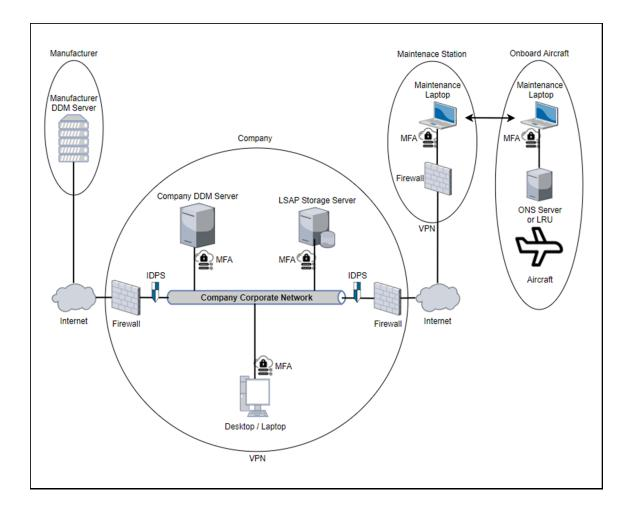
Figure 7. Security Architecture for LSAP Distribution System Source: Own - created using "Draw.io" app
