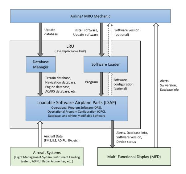
Figure 6. Detailed view of the LSAP and its interactions with the mechanic (*This figure refines the LSAP control structure further for STPA-Sec analysis*)
