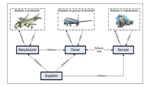
Figure 1. Airplane Assets Distribution System (AADS) Source: [10]
