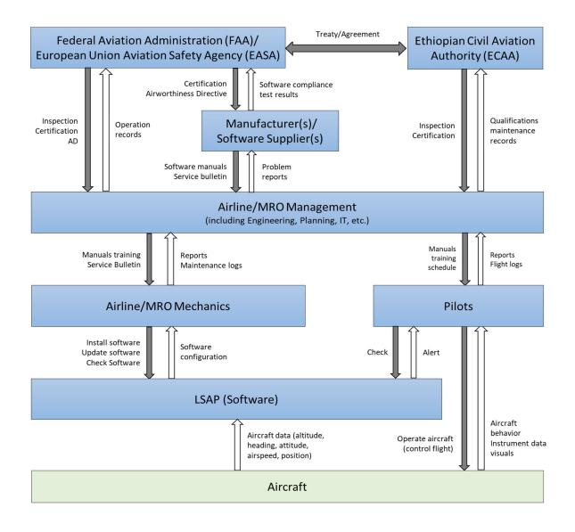
Figure 5. Control Structure for LSAP in airlines
