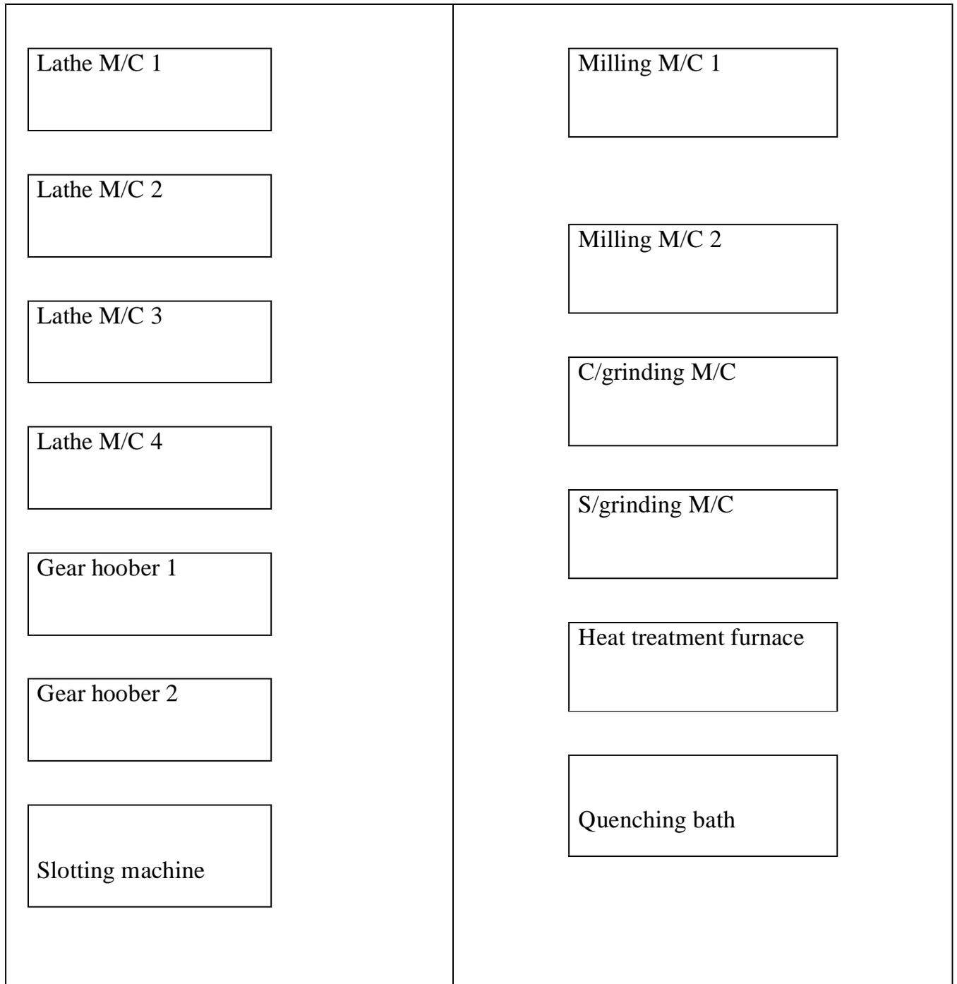
**Fig 3 Recommended Machine layout of gear manufacturing work shop**
